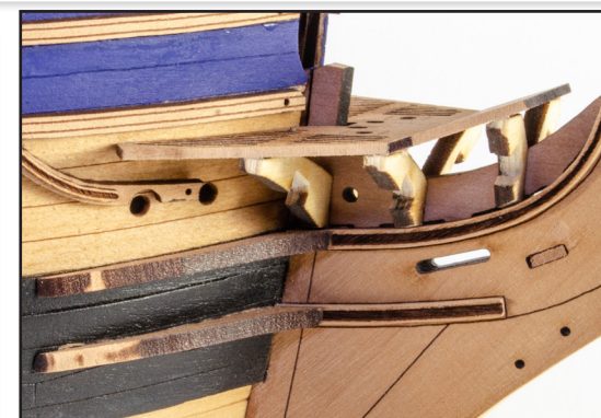
292. Glue the Bow Cheeks into position as shown. These will sit on top of the rails you recently fitted to the prow.
