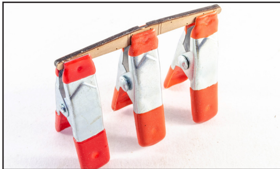
918. Glue each anchor stock side pattern to the relevant anchor stock, as shown. Note that the stock has an engraved centre into which the anchor will sit.
