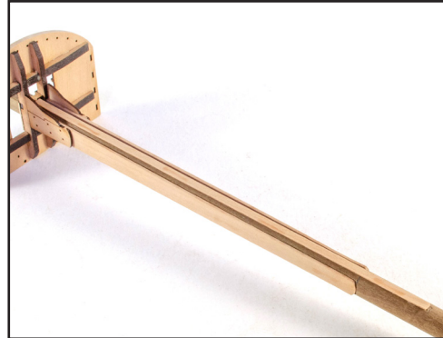
859. Glue the Front Fish into place on the front of the mast.
