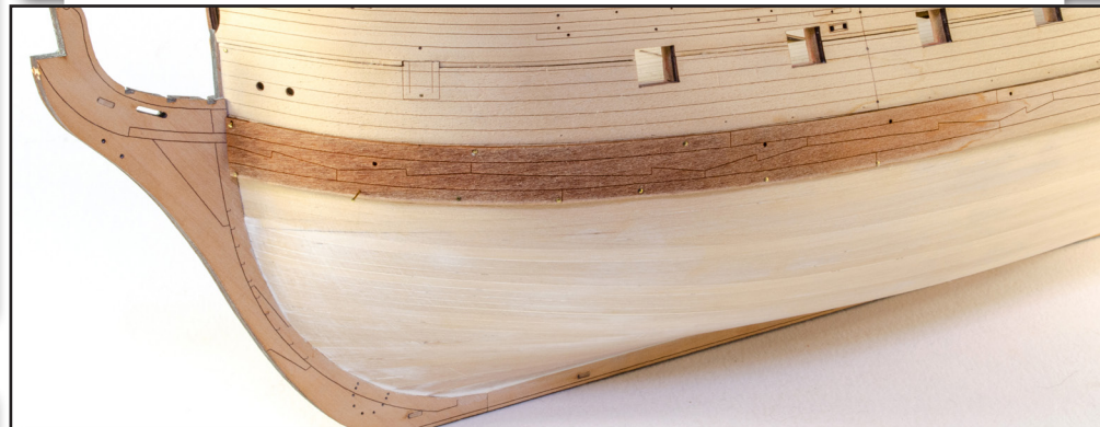
188. Take each of the main wale patterns and soak them in hot water for 30 minutes. Lie each one in position on the hull and pin it in place until dry. Due to the expansion of pear when wet, we suggest you leave these parts at least 24hrs before proceeding later gluing to hull.
