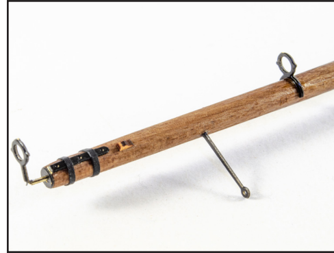
880. YARDS, GAFF etc: Make up all yards as per plans and don't forget the spritsail yards on the Mizzen/Bowsprit plan sheet. You can use either a cut-off brass pin to secure the yards to the masts, or brass wire. For the prototype, we have used the thicker wire option.
