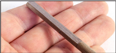
813. The mast sections will go through a number of shape changes to their cross section. Here you see the upper area of the lower section, squared-off on one side to fit the cross trees.
