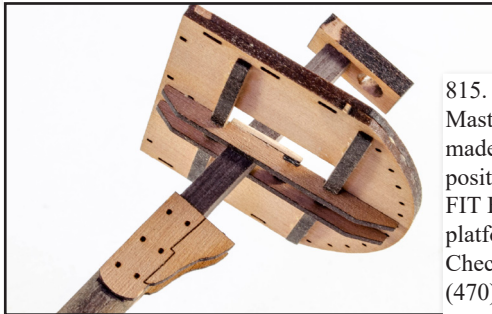
813. The mast sections will go through a number of shape changes to their cross section. Here you see the upper area of the lower section, squared-off on one side to fit the cross trees.
