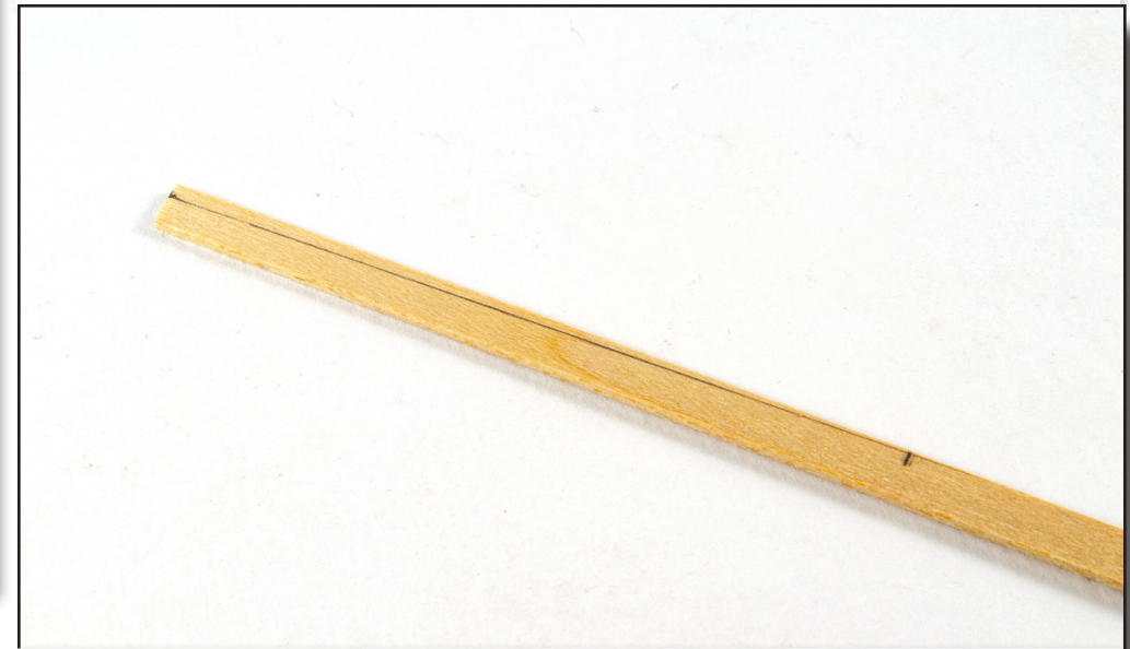
139. Now make another pencil mark about 1/3 to 1/2 down front end of strip and cut between the two marks, seen here in pencil. NOTE: on my prototype, I didn't find a need to taper the stern end of the plank, only the bow.
