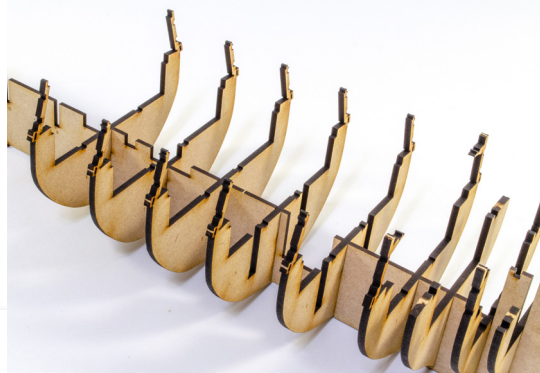
29. Slot bulkheads 1-1, 2, 2-2, 3 and 4 into position. Handle these gently as mishandling could damage the ears. Do NOT glue at this time.
