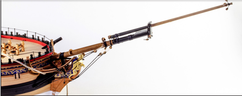
878. Glue bowsprit into position at bow, making sure the orientation is correct and it runs perfectly in line from bow to stern.
