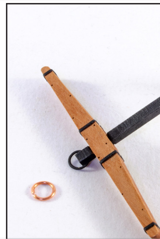
922. Use some brass wire to form the anchor hoops. Fit these to the anchors and paint black.
