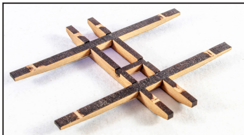
851. Assemble as shown. You can also shape the bolsters and glue them into position as on the other masts.
