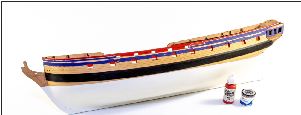
236. Varnish all of the hull above the waterline, except for the areas where the rail sections and channels will be glued. Now paint blue and red into their respective areas. You may need a couple of coats to achieve a good finish. We use Humbrol 25 Flat Blue enamel and Vallejo Flat Red acrylic for this.
