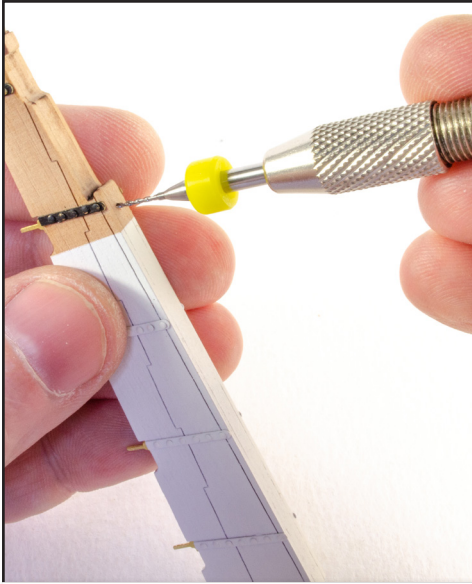
259. Push into place on the rudder so the pin makes a mark on the rear of the rudder. Remove the part and drill into the rudder using a 0.6mm drill, in the marked position.
