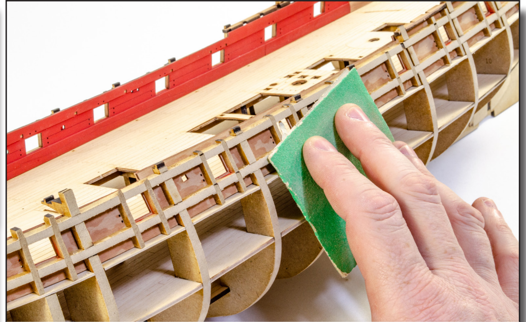
128. Before adding any jigs, it's time to fair the hull in readiness for planking etc. Most of the hard work is already done at the bow and stern, and they will only need a little extra sanding. Sand the hull so the lines flow properly and use a plank to lie against it at various points to ensure maximum bulkhead contact.
