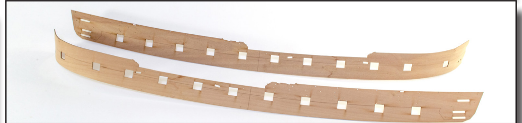
134. When removed from the hull, both parts will retain their curve and be easy to finally fit.
