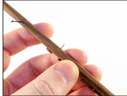
880. YARDS, GAFF etc: Make up all yards as per plans and don't forget the spritsail yards on the Mizzen/Bowsprit plan sheet. You can use either a cut-off brass pin to secure the yards to the masts, or brass wire. For the prototype, we have used the thicker wire option.
