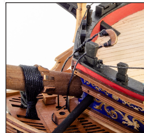
891. Slot the rigging cord through the round holes in the bow grate and then through the hole in the bow knee. You can seize both ends of this together (either above or below the grate, so the block is in the position shown on the plan. This can also be seen on Plan Sheet 21.
