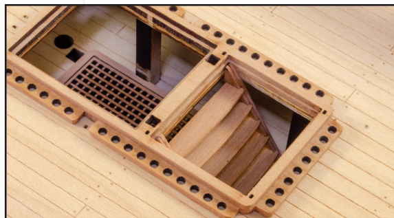
370. The ladder can now be glued into position as seen here.
