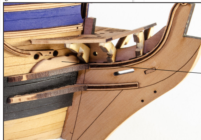
291. The Bow Cheeks will need a little beveling where they meet the hull and the prow. Check your beveling so ensure a good fit.
