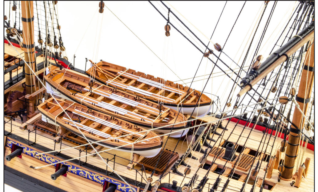
913. The beams and ship's boats are now fitted, and the Main Stay and Fore Hatch Tackle lashed down to them. The tackle hook can be secured to a boat lashing, and the other end to a beam.
