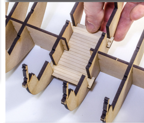
33. Making sure the bulkheads are fully seated, glue the orlop into position between bulkheads #4 and #5. Leave to dry.
