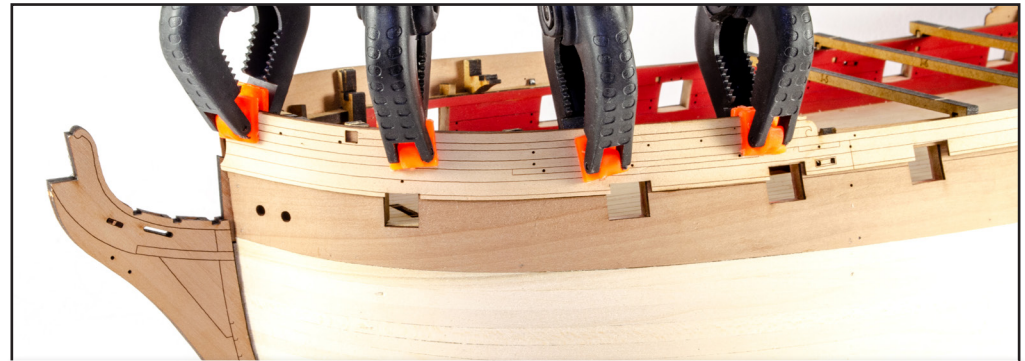
163. Soak these parts for 30 minutes in hot water and then clamp in position on the hull, until completely dry. We suggest leaving this overnight, for a minimum of 12hrs as pear can expand quite a lot when soaked.
