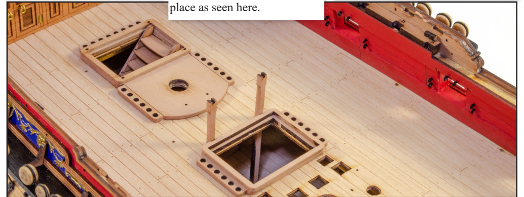
373. Bend the PE parts and sit on top of the stanchion. Now drill through the PE part into the stanchion (all the way through). Remove the PE part.
