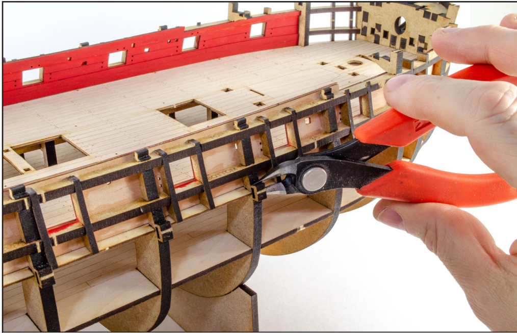
121. As the basic hull structures are now complete, we need to fair the hull in preparation for planking. Before we can do this, the 'safety gates' must be snipped from each of the bulkheads along the gun deck height, as seen here. The hull is now very strong and no longer needs these features.
